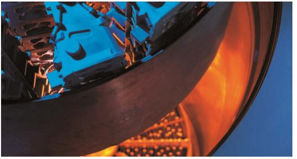
A high temperature furnace inside a pressure vessel
