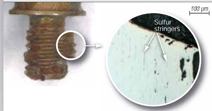
Fig. 1 a-b: Material, AISI 303 (1.4305); Left: Surface hardened bolt shows rust after usage in chloride-containing environment; Right: High amount of sulfur stringers in the material microstructure leads to a reduced corrosion resistance in aggressive media.
