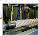
■The rotor must be finish polished using diamond tools due to the extreme hardness of the ceramic treatment
