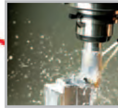
The injector is rough machined to within tight tolerance of its final size, adding fuel ports and passageways.
