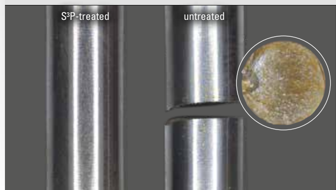
Fig. 3 Ten times improved fatigue life of S 3 P-treated sample AISI 316L (1.4404), also under corrosive load (5 wt. % NaCl-solution, < 35 °C, 400 MPa bending load, 15 Hz). No failure even after over 10 million cycles.
