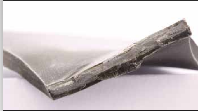
Fig. 1 Fatigue fracture of a propeller blade (AISI 304, 1.4301).
