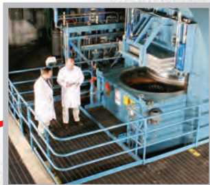
The implants are then HIPed to eliminate porosity, improve fatigue life and enhance the bonding of the biocompatible coating.
