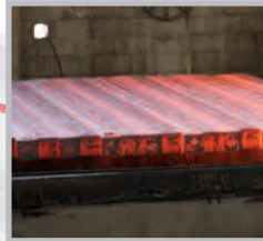
The gears begin life as low alloy steel.
