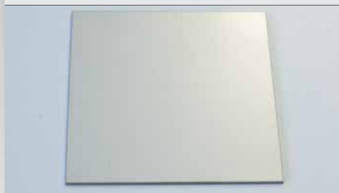
Fig. 2 Tested specimen; AISI 316L sheet metal (as-rolled 2B surface) after Kolsterising®.
