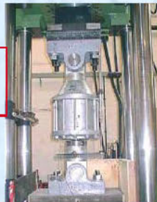
Testing bridge damper
