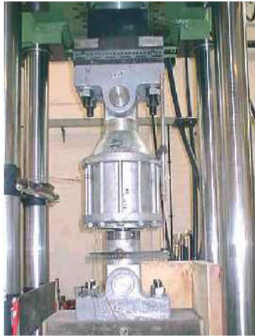
High load test on bridge damper
