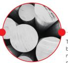
The watch case begins its journey as a steel billet. An austenitic stainless steel with high nickel and chromium content is selected for its non-magnetic properties and corrosion resistance. Quality and purity of the steel is critical to guarantee functionality and an optimal surface.
