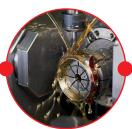
The case – a complex 3D shape – is machined from a disc or circular blank to tight tolerances, to meet the demands of specification and functionality.\*
