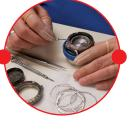
The individual watch components – up to 300 parts – are manually assembled.\*
