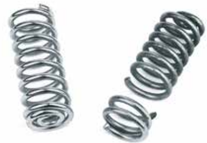
Fig. 1 Unused spring (left). Aged and fractured spring (right).
