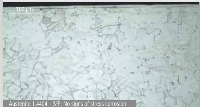
Austenite 1.4404 + S 3 P: No signs of stress corrosion
