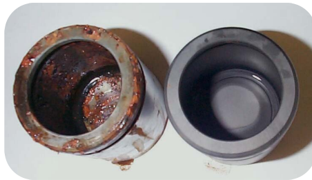
60hr salt spray test vs chemical coatings
