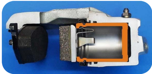
Brake piston (280gm v prior 440gm)
